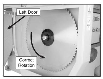
**Figure 31.** Checking blade rotation from left door.
